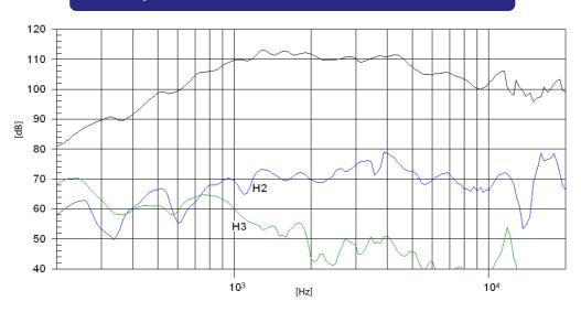
**Note:** On axis frequency response measured coupled to TD-365 horn in anechoic chamber, 2,83 v @ 1m
